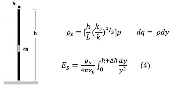
Fig. 2. Electric field  $E_S$  at  $S$ , caused by an upward leader.
