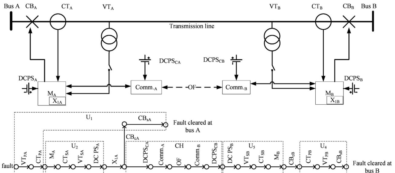
**Fig. 1.** Single distance protection with single aided communication channel—reliability and reliability graphs of the fault clearance process triggered by the Bus A distance protection (tie-set<sub>2</sub>).
