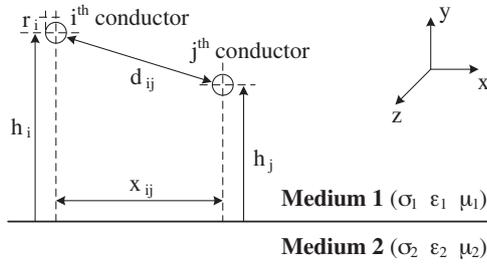
Fig. 1. Multiphase conductor arrangement.
