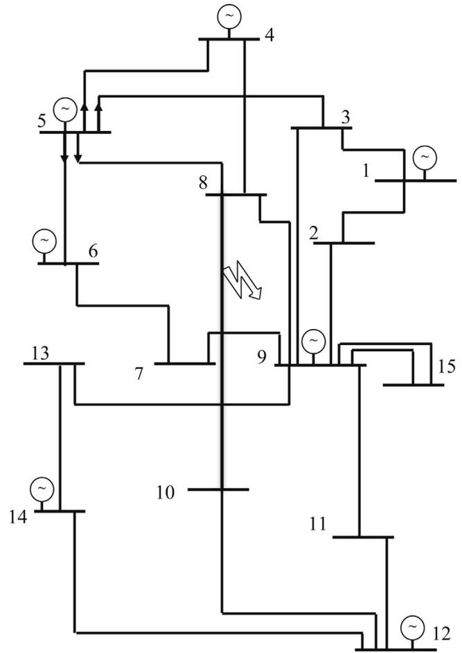
Fig. 1. Single-line diagram of a sample faulted network.
