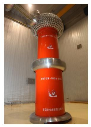
Fig. 3. The 1000 kV adjustable frequency transformer.
