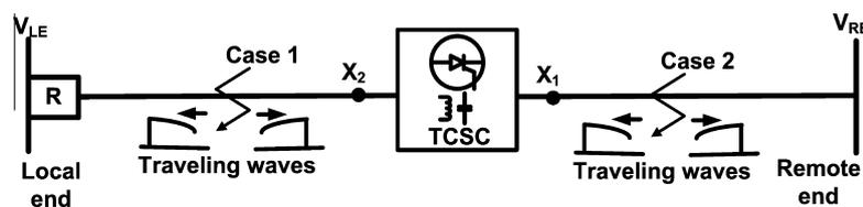
Fig. 1. Traveling waves during two fault events.
