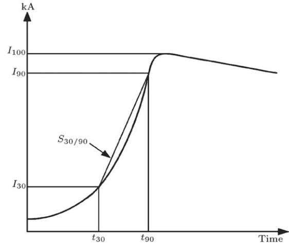
Figure 1: Typical return stroke waveform of lightning current.
