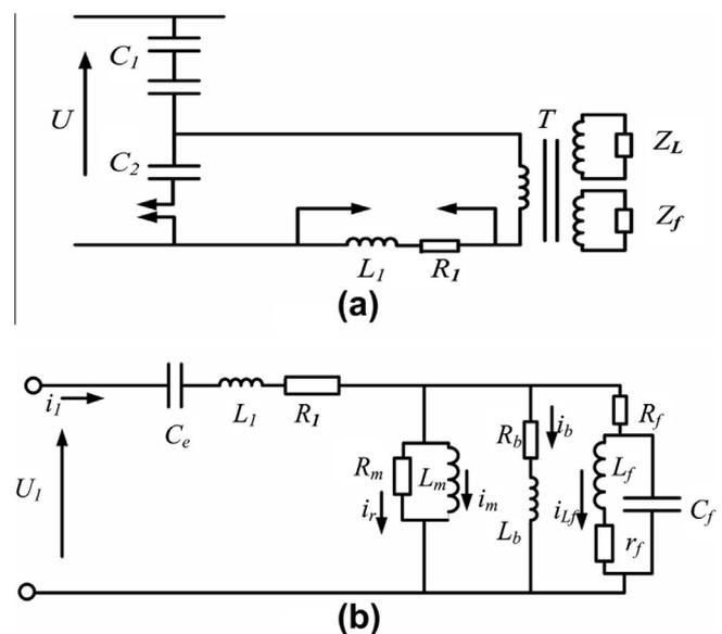
Fig. 1. CCVT circuit: (a) actual circuit; (b) equivalent circuit.
