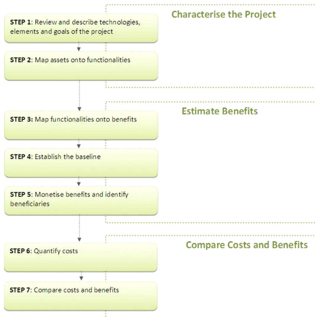
Fig. 1. General framework of the cost benefit analysis performed in GreenLys and developed by the European Commission [1].
