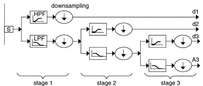
Fig. 3. Three-level DWT.
