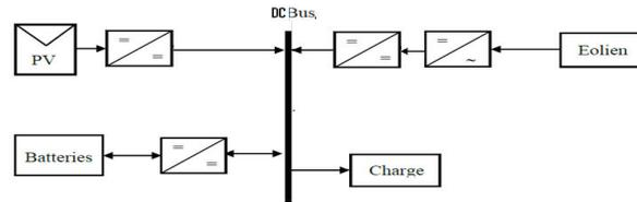
Fig. 1. Multi-source system architecture developed in this work
