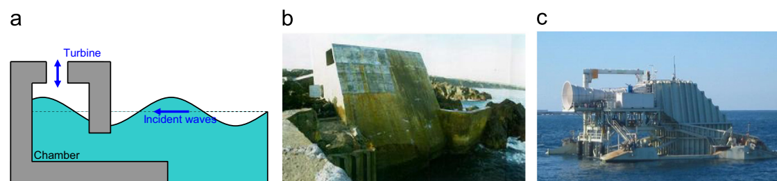
Fig. 2. Oscillating Water Column devices: (a) schematic; (b) Pico shore-based OWC built in the Azores in 1999; (c) Oceanlinx floating OWC deployed in 2010 in New South Wales, Australia.
