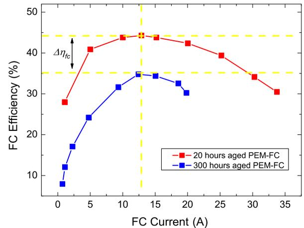
Fig. 1. Efficiency curves for two PEM-FCs with different degrees of degradation at  $T_{fc} = 35^\circ\text{C}$ .
