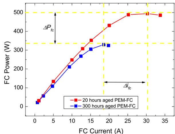
Fig. 2. Power curves for two PEM-FCs with different degrees of degradation at  $T_{fc} = 35^\circ\text{C}$ .
