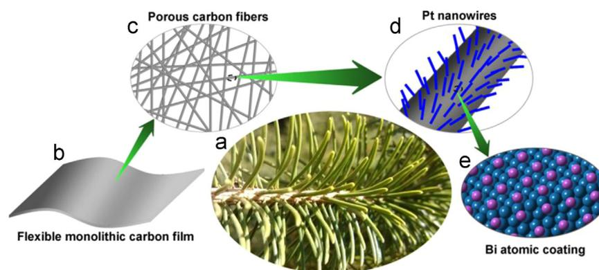
**Figure 1** Hierarchical structures in nature and by design. (a) Optical photo of a branch showing the hierarchy wire on wire structure of a pine tree. (b-e) Monolithic thin film catalyst composed of porous carbon nanofibers on top of which Bi decorated Pt nanowires were grown.
