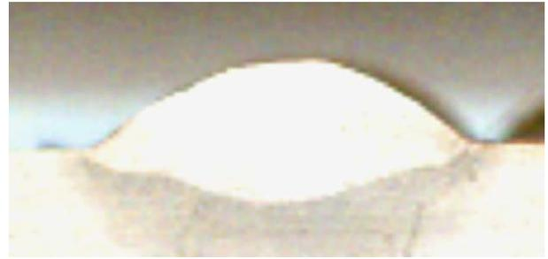
Fig. 1. Micro-photograph of a sectioned bead geometry.
