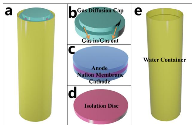
Fig. 2. Schematic of the fuel cell-type sensor (a), which is composed of (b) a gas diffusion cap, (c) the MEA, (d) an isolation disc and (e) a water container.
