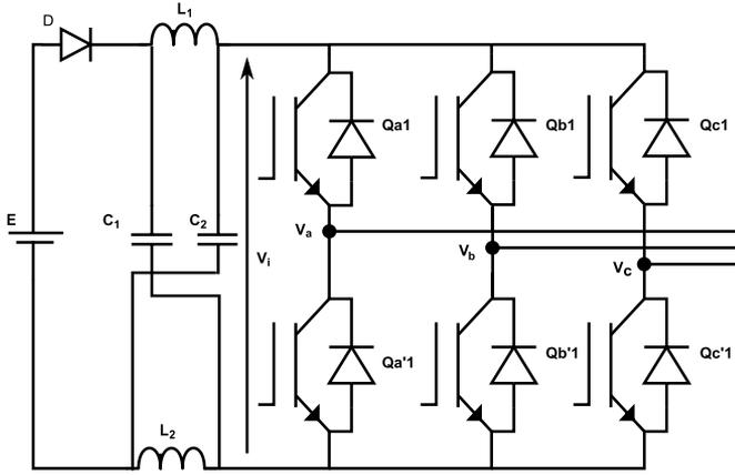
Fig. 1. Topology of two-level Z-source inverter.
