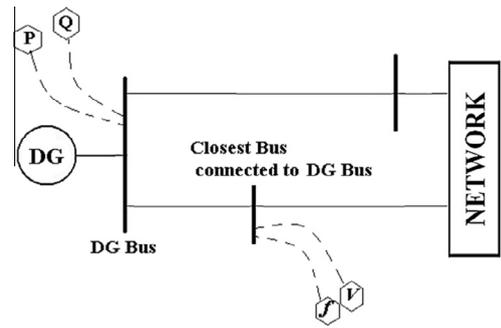
Fig. 3. Configuration of multivariable islanding detection method.
