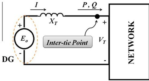
Fig. 1. Equivalent circuit of network with DG unit.
