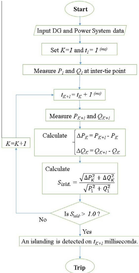
Fig. 2. Flowchart of the first proposed method for islanding detection.
