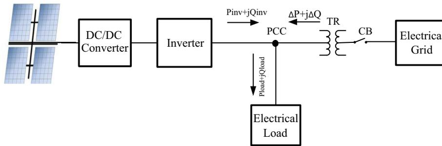
Fig. 2. Islanding in a PV-based DG system.
