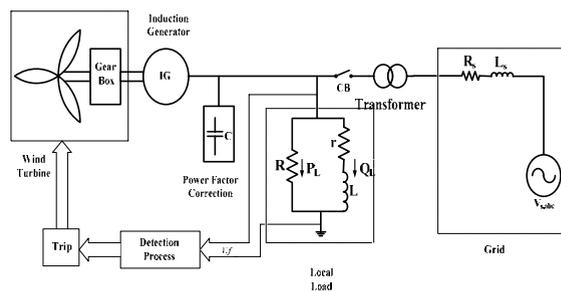
Fig.1 Test system to detect islanding conditions including a local load, a power grid and a wind turbine
