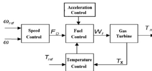
Fig. 1. Microturbine control system architecture
