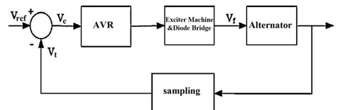
Fig. 2. Block diagram of the genset.
