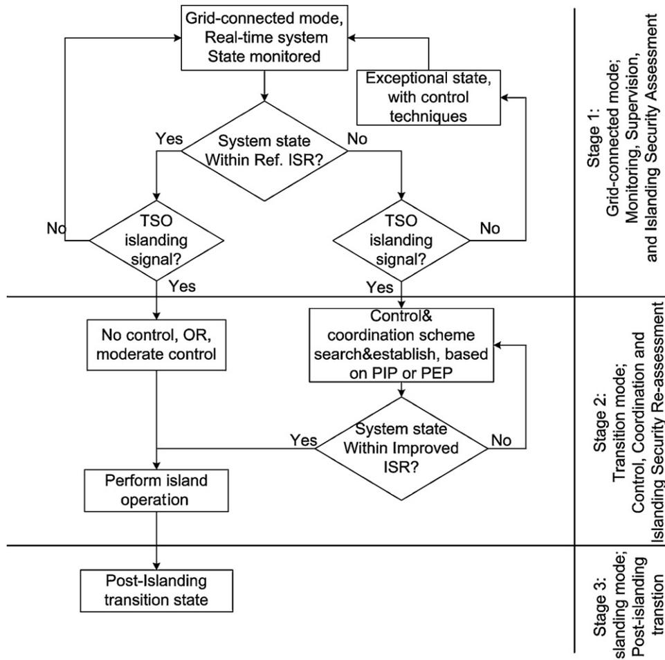
Fig. 1. Islanding Control Architecture for intentional islanding transition.
