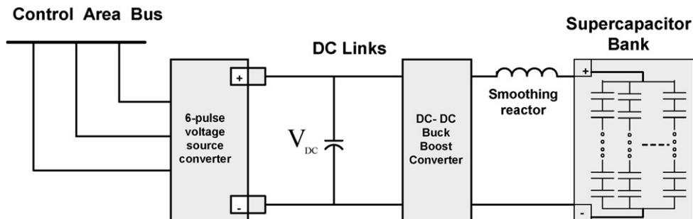
Fig. 2. Configuration of super-capacitor bank in control area.
