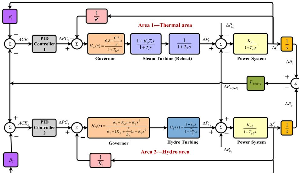
Fig. 1. Block diagram of a two-area interconnected hydrothermal power system.
