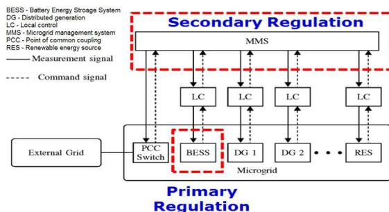
Fig. 1. hierarchical control structure
