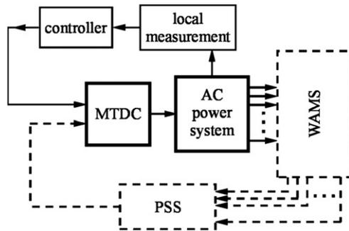
Fig. 2. Schematic illustration of a local control and a state-variable stabilizing control.
