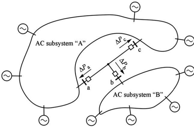
Fig. 1. Two subsystems connected by a MTDC network.
