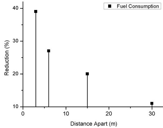
**Fig. 2.** Measurement results of fuel consumption at 89 km/h [21].
