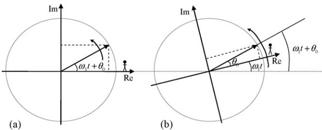
Fig. 2. Stationary reference frame (a) and rotating reference frame (b).
