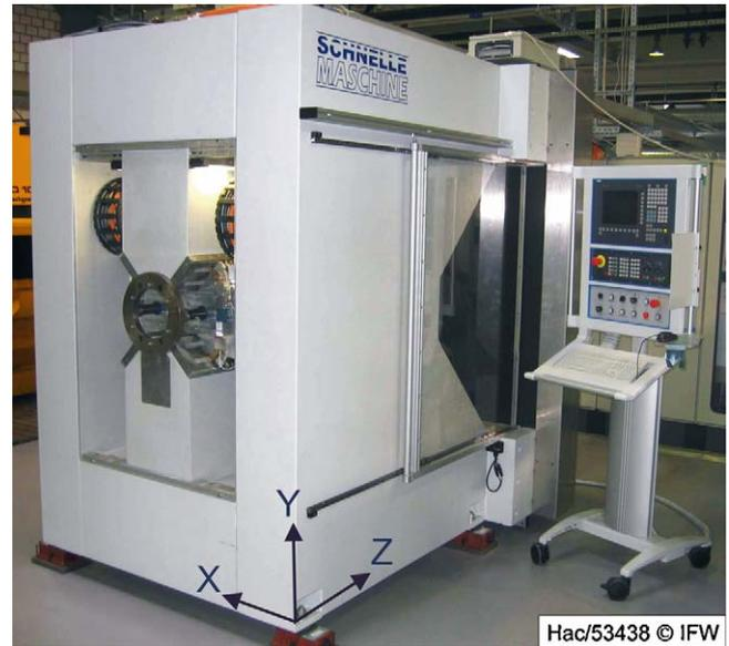
Fig. 1. Machine tool with active magnetic guides.
