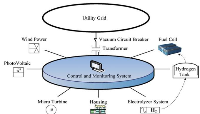
Fig. 1. System configuration of micro-grid network.
