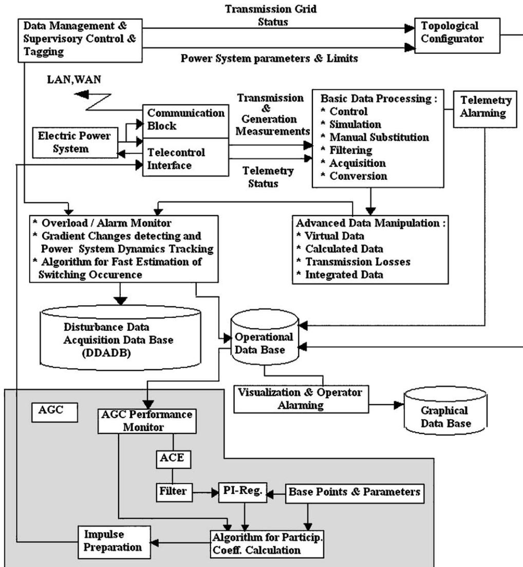
Fig. 1. Diagram of SCADA & AGC system.
