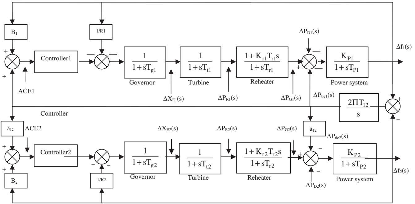
Fig. 1. Block diagram of Two Area Power System.
