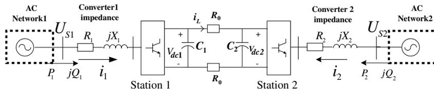
Fig. 1. Physical model of HVDC Light system.
