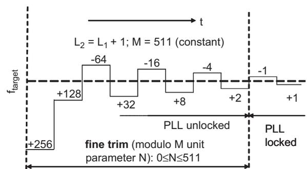
Fig. 4. Frequency acquisition and control scheme of DCO.
