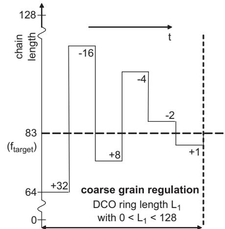
Fig. 3. Frequency acquisition and control scheme of the ring length tuning.
