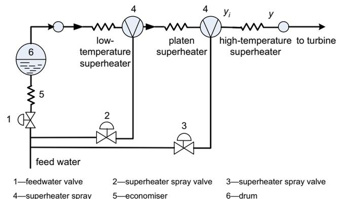
Fig. 2. Superheater process.
