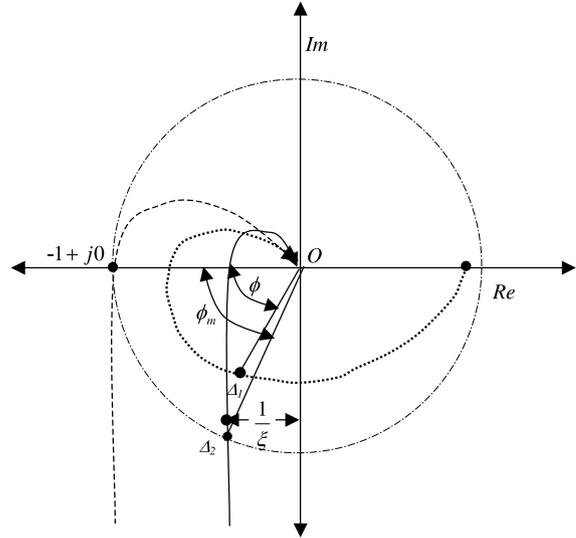
Fig. 2. Nyquist curves of the uncompensated process ( $\cdots$ ), the process with the modified relay ( $---$ ) and the process with the controller ( $-$ ).
