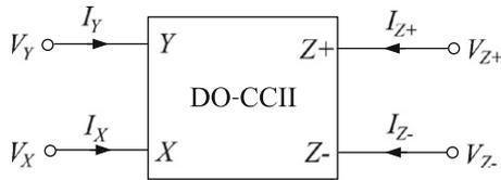
Fig. 1. Circuit symbol of the DO-CCII.
