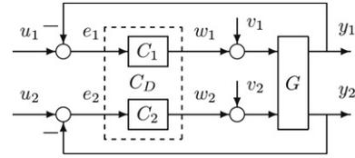
Fig. 1. The two-channel decentralized system  $\text{Sys}(G, C_D)$ .
