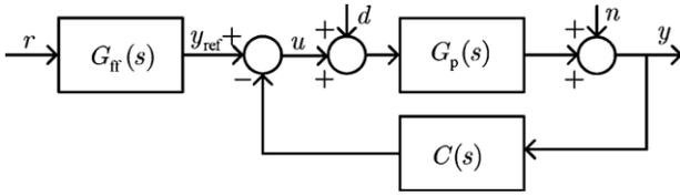
Fig. 1. Process  $G_p(s)$  with the controller  $C(s)$ .
