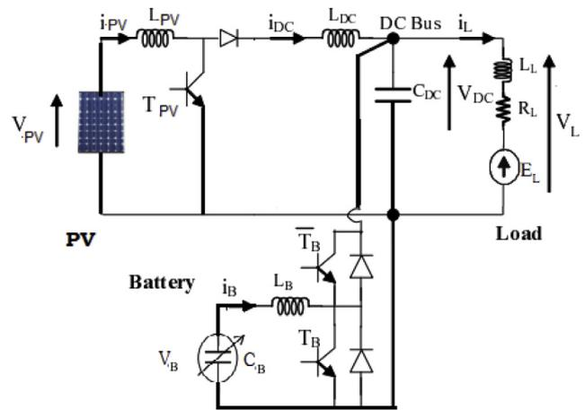
**Fig. 2 – PV/Battery hybrid system configuration.**
