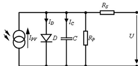
**Fig. 3 – Equivalent circuit diagram of a solar cell.**
