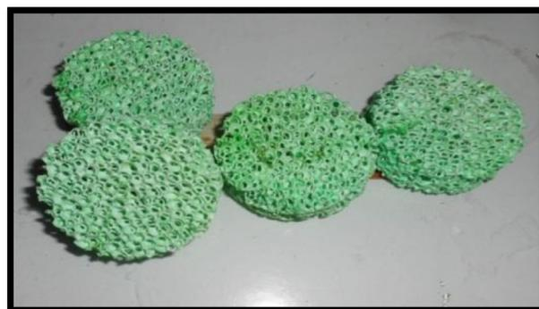
Fig. 1 – Alumina foam type catalyst with Ni coating.
