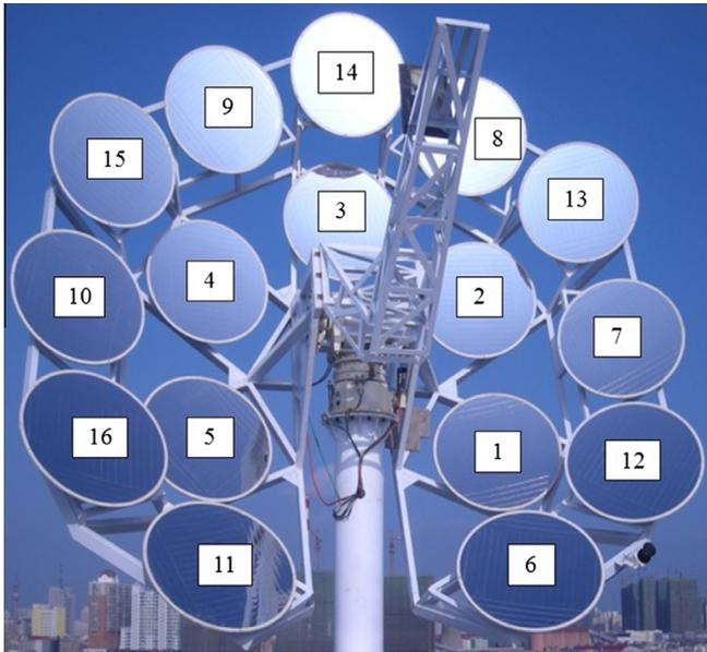
Fig. 1. Schematic diagram of the multi-dish solar concentrator system.
