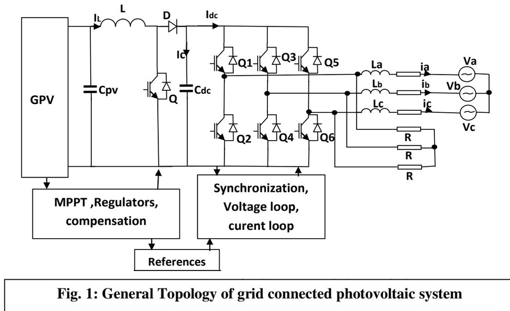
**Fig. 1: General Topology of grid connected photovoltaic system**
