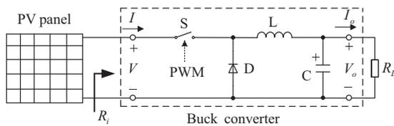
Fig. 2. Structure of PV system with buck DC/DC converter.
