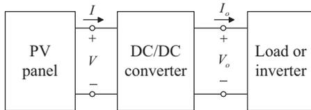
Fig. 1. Structure of common PV system.
