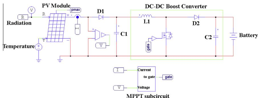
Fig. 1. Block diagram of a general PV system.
