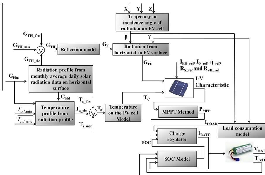
Fig. 1. Block diagram of the developed system.
