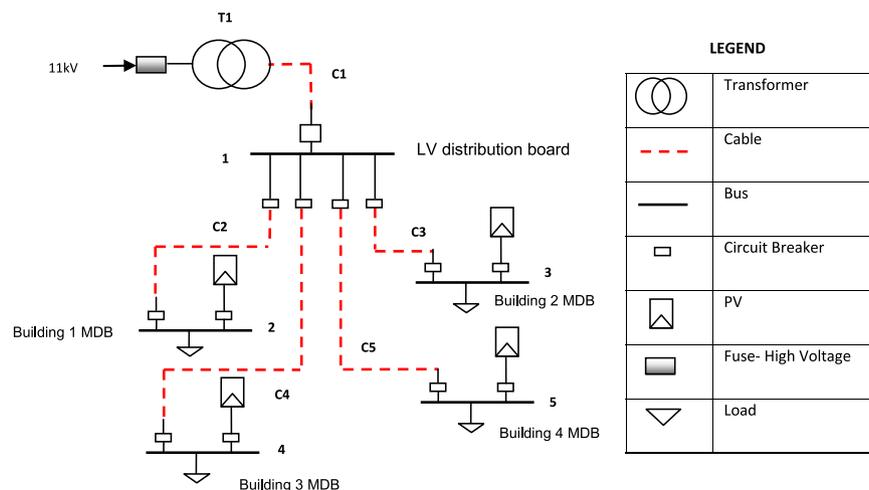
Fig. 1. Power distribution network – Power supply for buildings.
