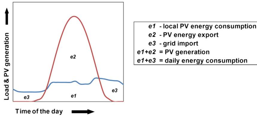
Fig. 1. The daily energy dynamics of a customer with a grid-connected PV system.
