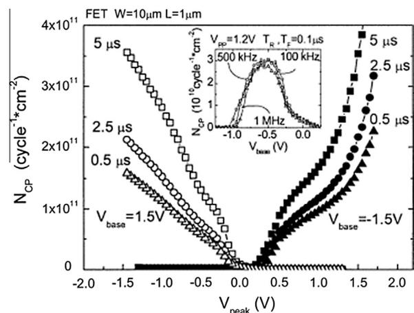
Fig. 2. Charge-pumping characteristics measured on n-channel MOSFET with a 3-nm deposited  $\text{HfO}_2$  layer. The conventional base level sweep (inset) is compared with the amplitude sweep using constant base level (after Ref. [19]).
