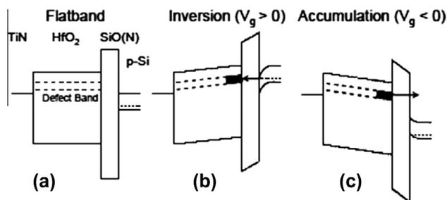
Fig. 1. Schematic energy-band diagram of a  $\text{SiO}_2/\text{HfO}_2/\text{poly-Si}$  gate stack containing a defect band in the  $\text{HfO}_2$  layer at flatband condition shown in (a). For (b) positive and (c) negative bias, the defects located near the  $\text{SiO}_2$  interfacial layer move rapidly with respect to the Fermi-level in the Si substrate. In schematic (b) electron traps are negatively charged and in schematic (c) electron traps are discharged (after Ref. [19]).
